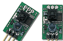
IR transmit and receive
