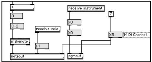
Figure 4-7: Velocity and the instrument informations are received from the random generator.
