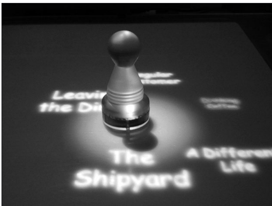
Fig. 62. Due to the strips at their base the pawns of Tangible Viewpoints can be sensed by the augmented 'playing' surface, thus enabling the projection of interactive images on the surface around the pawn. (image: MIT Image Laboratory)
