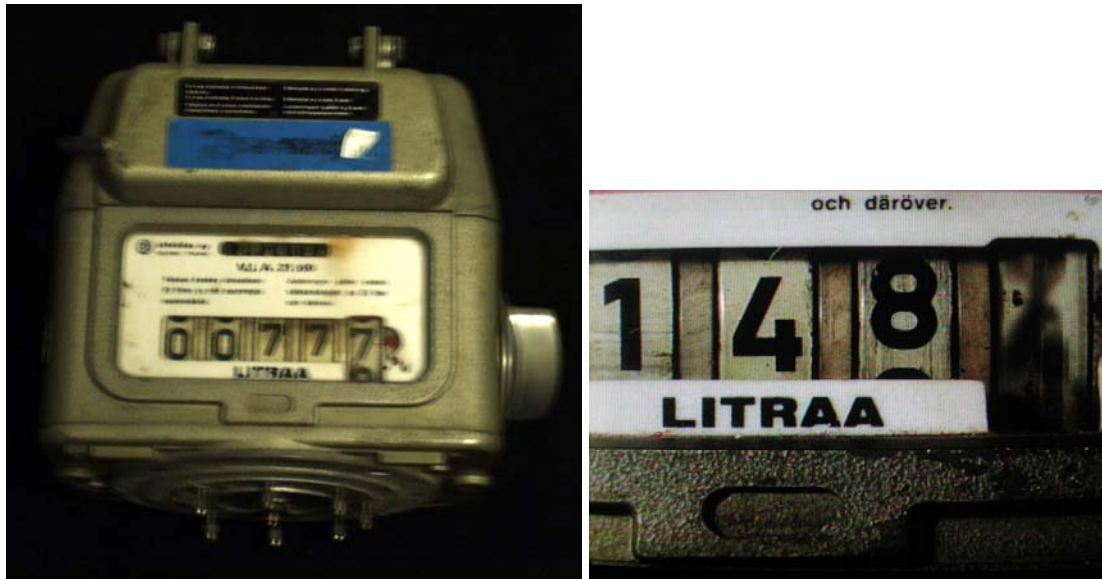
Picture 26. The milk machine's counter and its dials.
